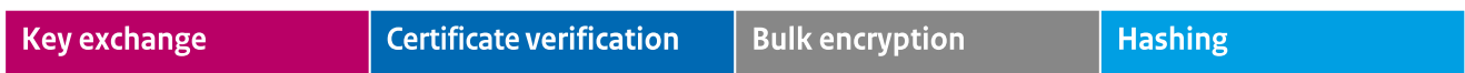
Figure 1 – Cipher suite notation in TLS 1.2 and TLS 1.3. The colours indicate the different algorithms and their purpose. In TLS 1.3, the cryptographic algorithms for key exchange and certificate verification are no longer considered part of the cipher suite.
