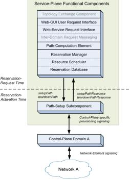
The functional components of NRPSs. Fenius is a solution for NRPSs that lack the highlighted inter-domain components. A better solution would be the standardization and integration of these components in NRPSs, enabling the exchange of topology information and status-notifications, and handle interdomain requests through a common interface.
