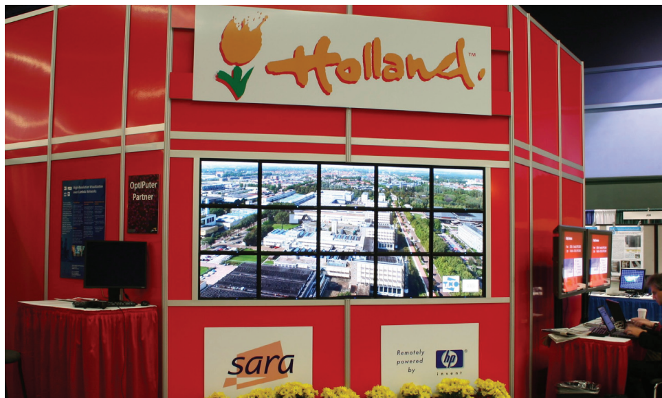
Fig 2.5.3: Tiled displays are used to create high resolution visualisation facilities. Here such a setup was demonstrated by SARA at SuperComputing 2005 in Seattle showing hi-resolution images from servers located in Amsterdam.
