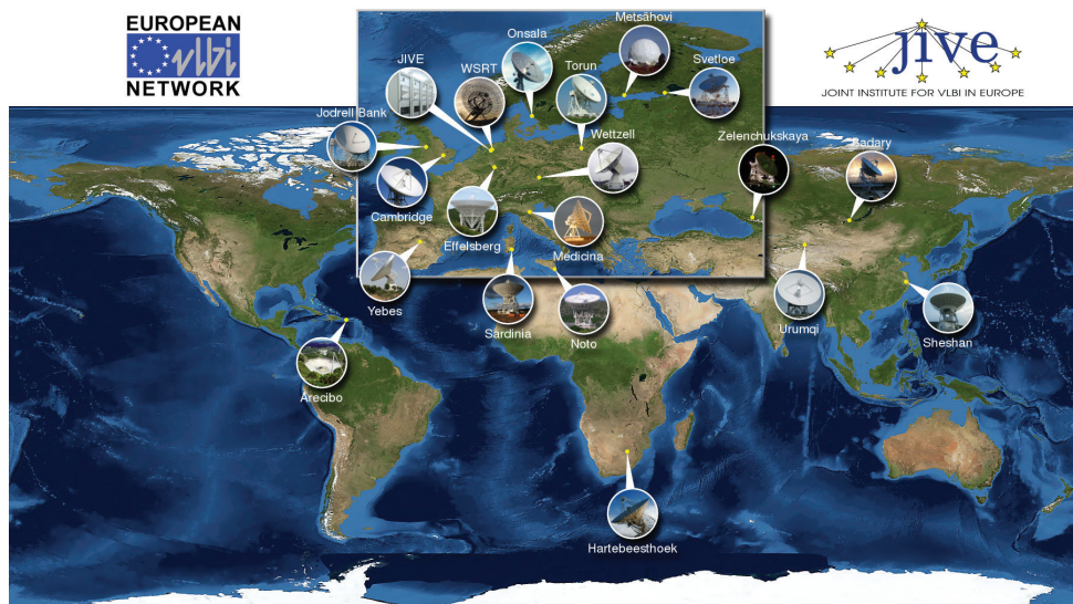
Fig 1.2 The European array of radio telescopes that require dedicated network connections allowing real-time correlation of signals from different telescopes to perform observations (Very Long Baseline Interferometry).
