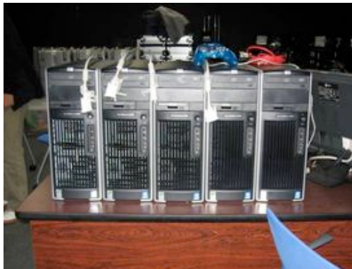
PC Cluster for real-time 4K rendering of Toppan's VR of the "Nijo Castle"
